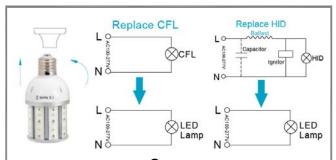
When installing Weihu LED® retrofit lamps within HID fixtures, ballast must be by passed when present. Our retrofits are UL damp rated;sealing the fixtures after installation will deliver best results. Installing surge/lightnig protectors is highly recommended and helps to eliminate premature driver failure caused by surges and other power fluctuations.
